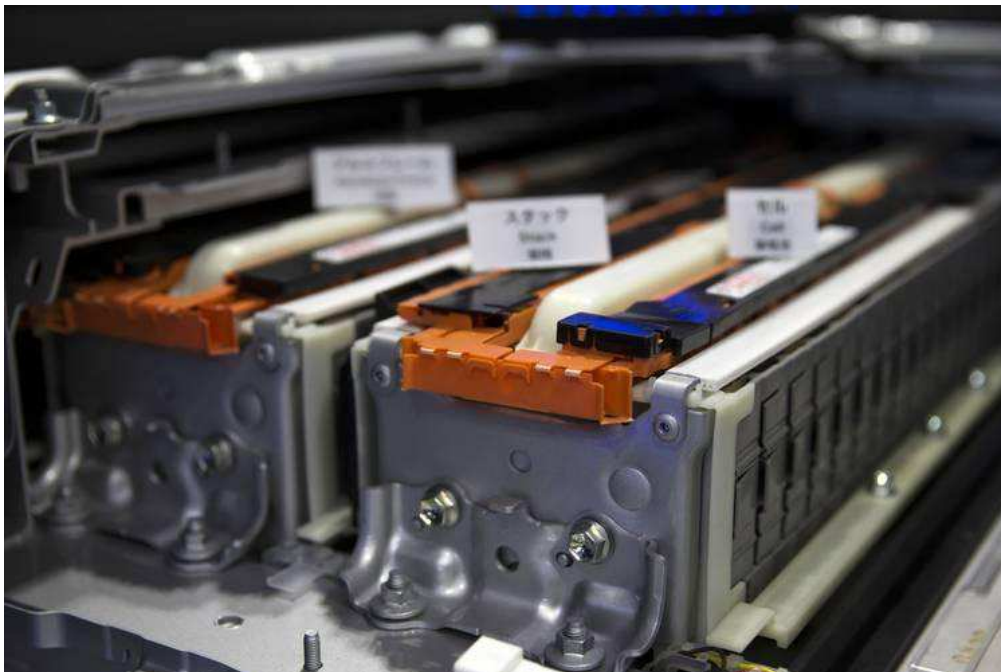
Lithium-ion batteries for Toyota's new Prius plug-in hybrid vehicle are on display. PHOTO: TOMOHIRO OHSUMI/BLOOMBERG NEWS
