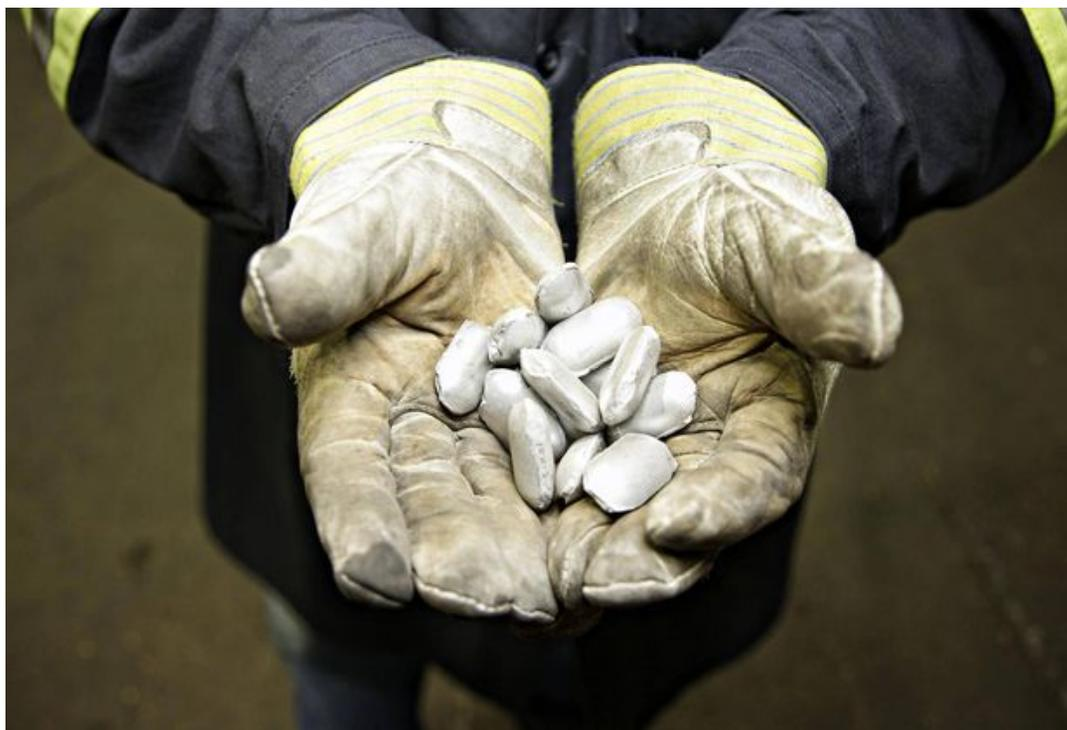
Cobalt briquettes produced at Sherritt International's refinery in Fort Saskatchewan, Alta. The hard, lustrous, grey metal is used in the production of high-temperature and wear-resistant super alloys, magnetic alloys, rechargeable batteries and chemicals.
