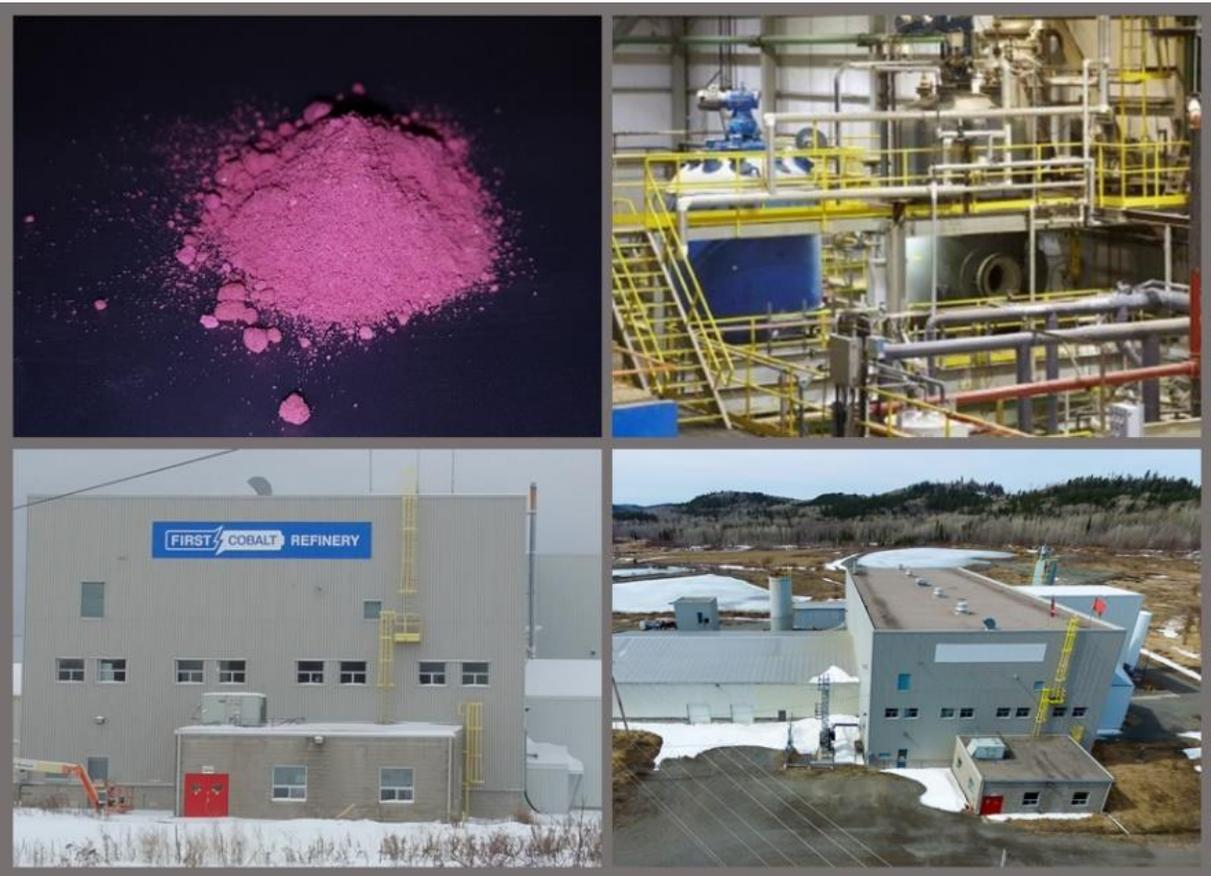
**Image 1. Top left to right, cobalt sulfate produced using the First Cobalt Refinery flowsheet; current autoclave circuit. Bottom left to right, external and aerial images of the facility.**
